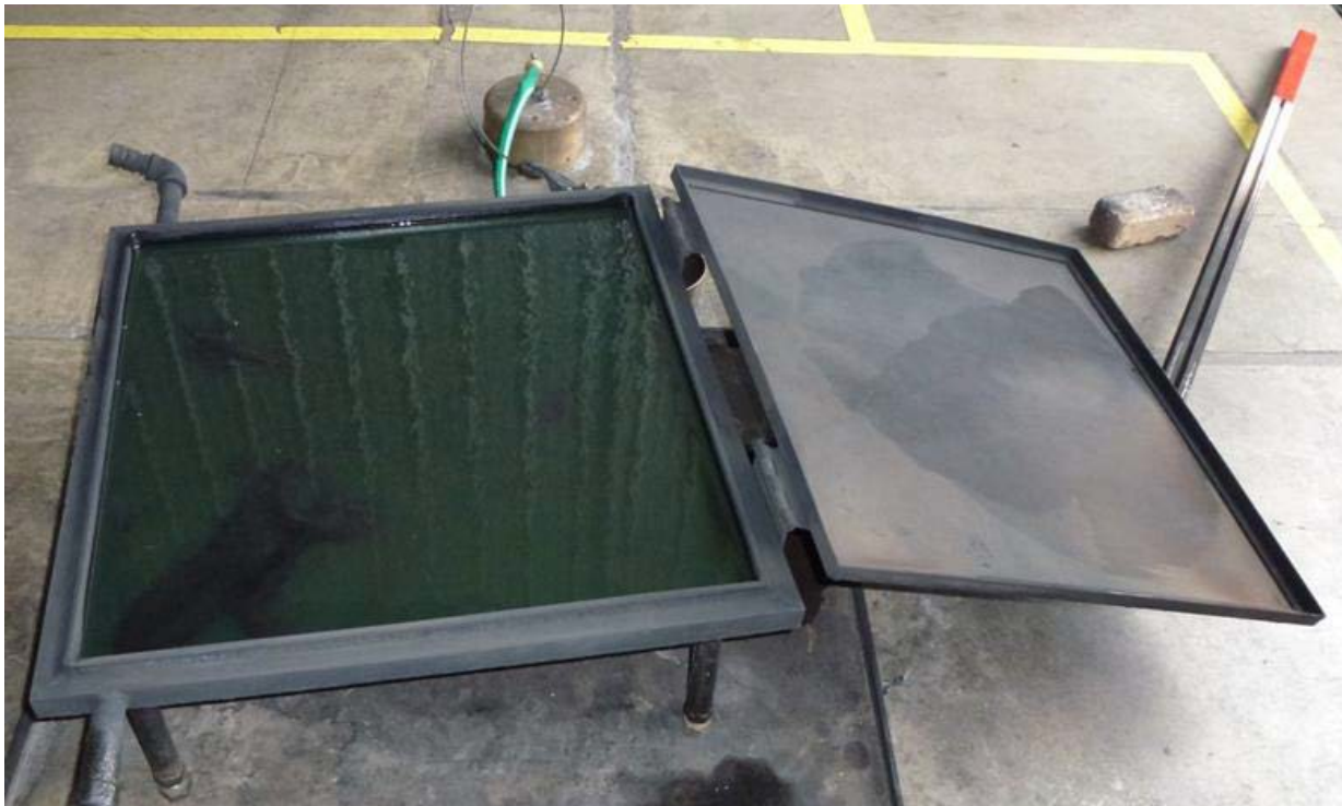
Figure E-17: Example of Fire Pan, for Acceptance Test of Optical
