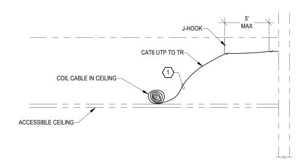
NOTE: WIRELESS ACCESS POINT AND ANTENNA NOT IN CONTRACT. DETAIL NOTE: 1 COIL 20' LOOP IN CEILING.
