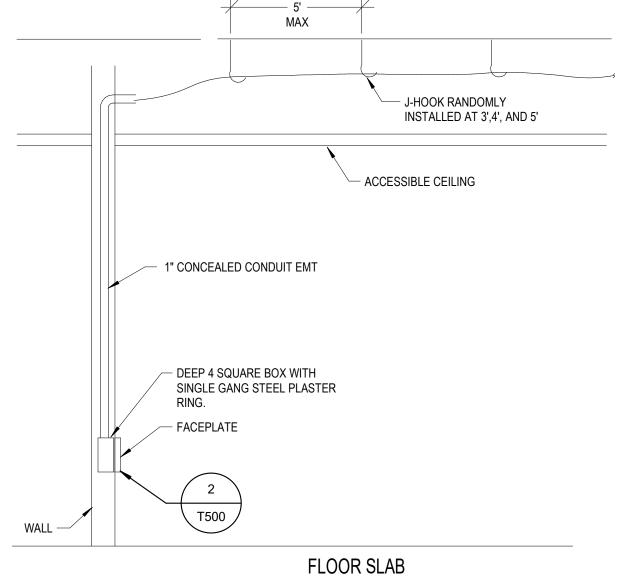
TYPICAL FLUSH MOUNT OUTLET (CONCEALED 3 <u>CONDUIT</u>)
