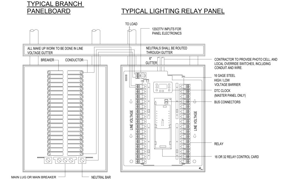
NOTE: COORDINATE CONTROL ZONE & SWITCHING LAYOUT WITH OWNER PRIOR TO PROGRAMMING & INSTALLATION.
